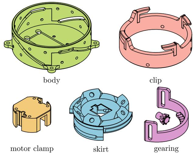
Fig. 2: The components of the connector
