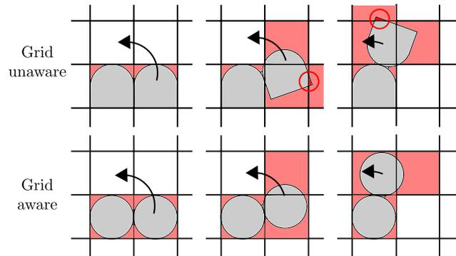
Fig. 3: Illustration of grid awareness. If a double cell modules tries to move one of its bodies from right to top, grid-unaware module occupies extra cells of the grid.
