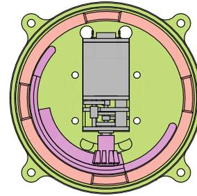
Fig. 7: Internal arrangement of the connector – top view without skirt. The motor is shown gray.
