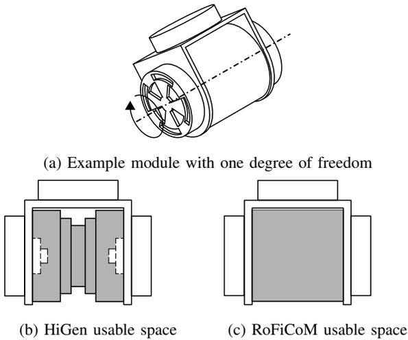
Fig. 6: Comparison of usable body space (gray) of an example module for the HiGen and RoFiCoM connectors
