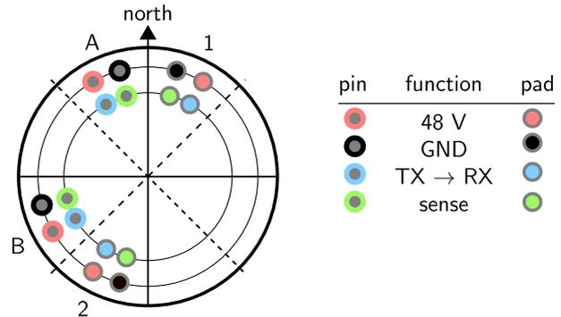
Fig. 8: Skirt pins arrangement allowing for 90-degree symmetric connection
