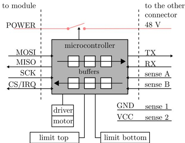
Fig. 9: Block diagram of the connector.
